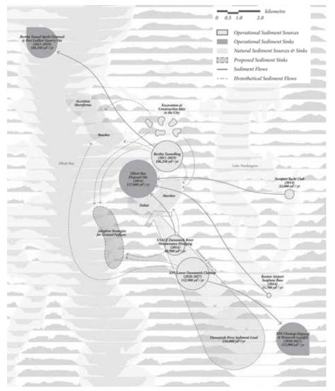
Figure 6. Annual sediment flows, sources and sinks for natural processes and earthwork operations in the Puget Lowlands.
