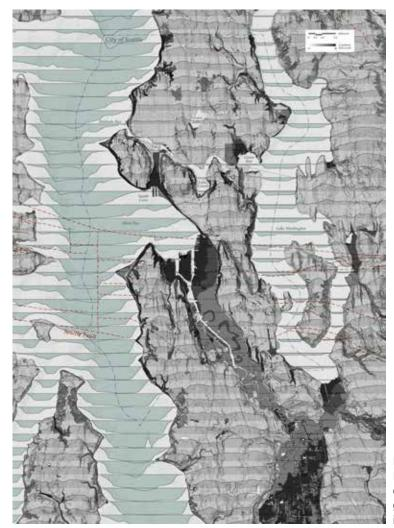
Figure 1. Risk zones of combined ground failures in Seattle.
