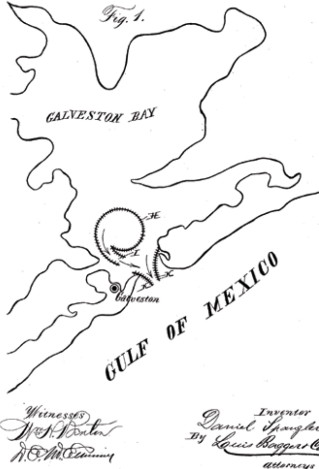
Figure 9. Invented in Hanford, California (1885), Daniel Spangler’s patent for a “Submarine Wall” imagines a subsurface louvered wall that focuses tidal power to self-dredge navigable channels. The system harnesses the hydraulic power of tidal exchange to passively dredge shallow bay bottoms such as those found in the San Francisco and Galveston Bay. The patent is also significant for its use of cartographic drawings that suggest a regional, or territorial, scale for technological innovation.
